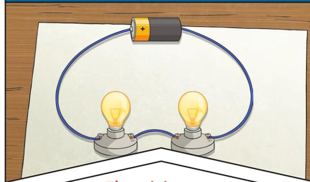
**Electricity** can only flow around a complete **circuit** that has no gaps. There must be wires connected to both the positive and negative end of the power supply/**battery**.
